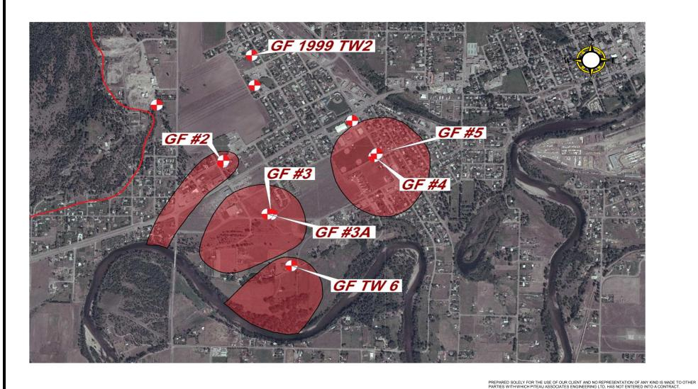
Capture Zones determined using Modflow model developed by Dr. D. Allen at Simon Fraser University (Allen, 2004)
