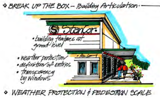
Figure 4.2: Weather Protection from Awnings
