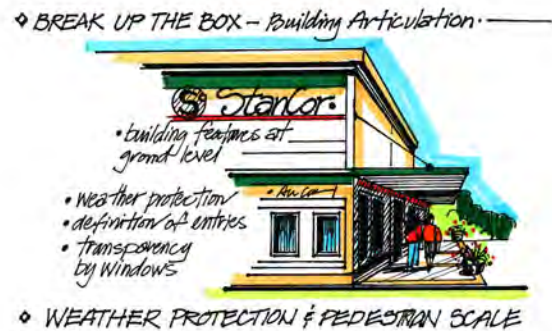
Figure 3.2: Weather Protection from Awnings
