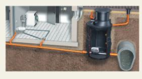
Installed on sewer services, permits operators to easily see whether a blockage is in the service line or sewer main, decreasing time spent troubleshooting.
