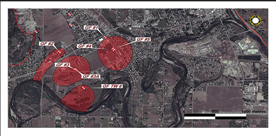
Capture Zones determined using Modflow model developed by Dr. D. Allen at Simon Fraser University (Allen, 2004)
